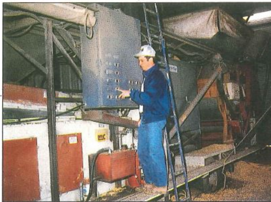
The portable seed cleaner is built on the bed of a semi-trailer.
